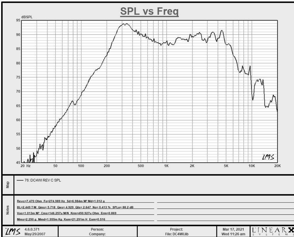
**TECHNICAL NOTE:** Sensitivity is measured with 2.83 volt input, measured on-axis at 1 meter distance
